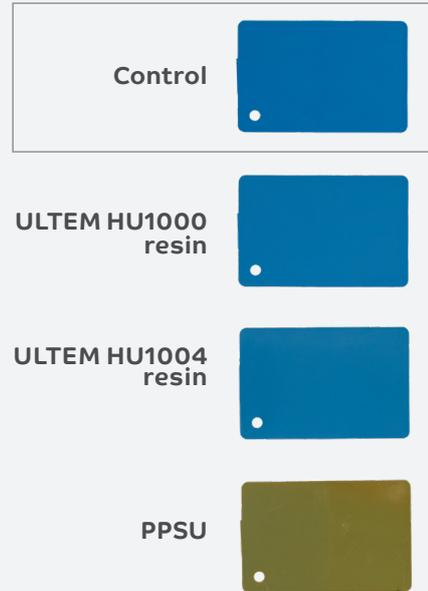
ULTEM HU1000 and HU1004 resins show minimal color change while the PPSU color deteriorates to a dark greenish hue and embrittles after 300 sterilization cycles. ULTEM resin can help your parts maintain their color and aesthetics even after repeated sterilization cycles.
