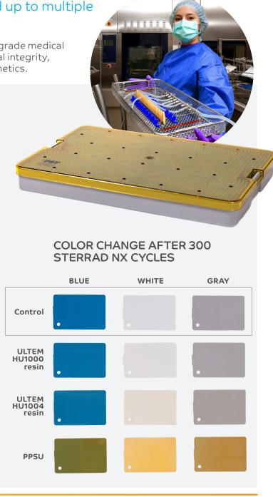
**ULTEM™ HU resins maintain mechanical properties** even after 300 VHP sterilization cycles. The PPSU material becomes embrittled and can break easily upon impact.
