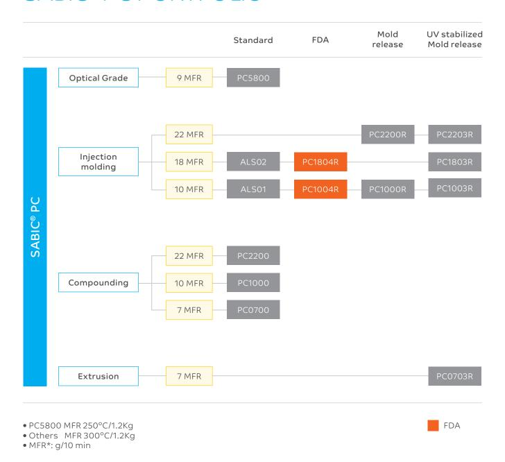
The SABIC® PC resin portfolio offers an optimized set of products designed to serve high volume applications in the extrusion, injection molding and optical media markets. We also offer a wide range of products for the custom compounding market.
