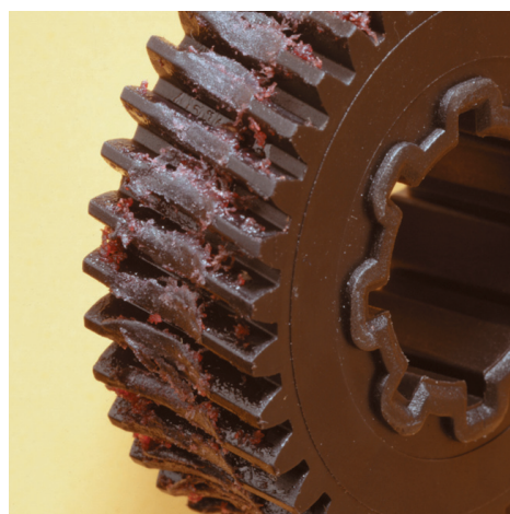
FIGURE 28 TOOTH DEFORMATION DUE TO EXCESSIVE HEAT
