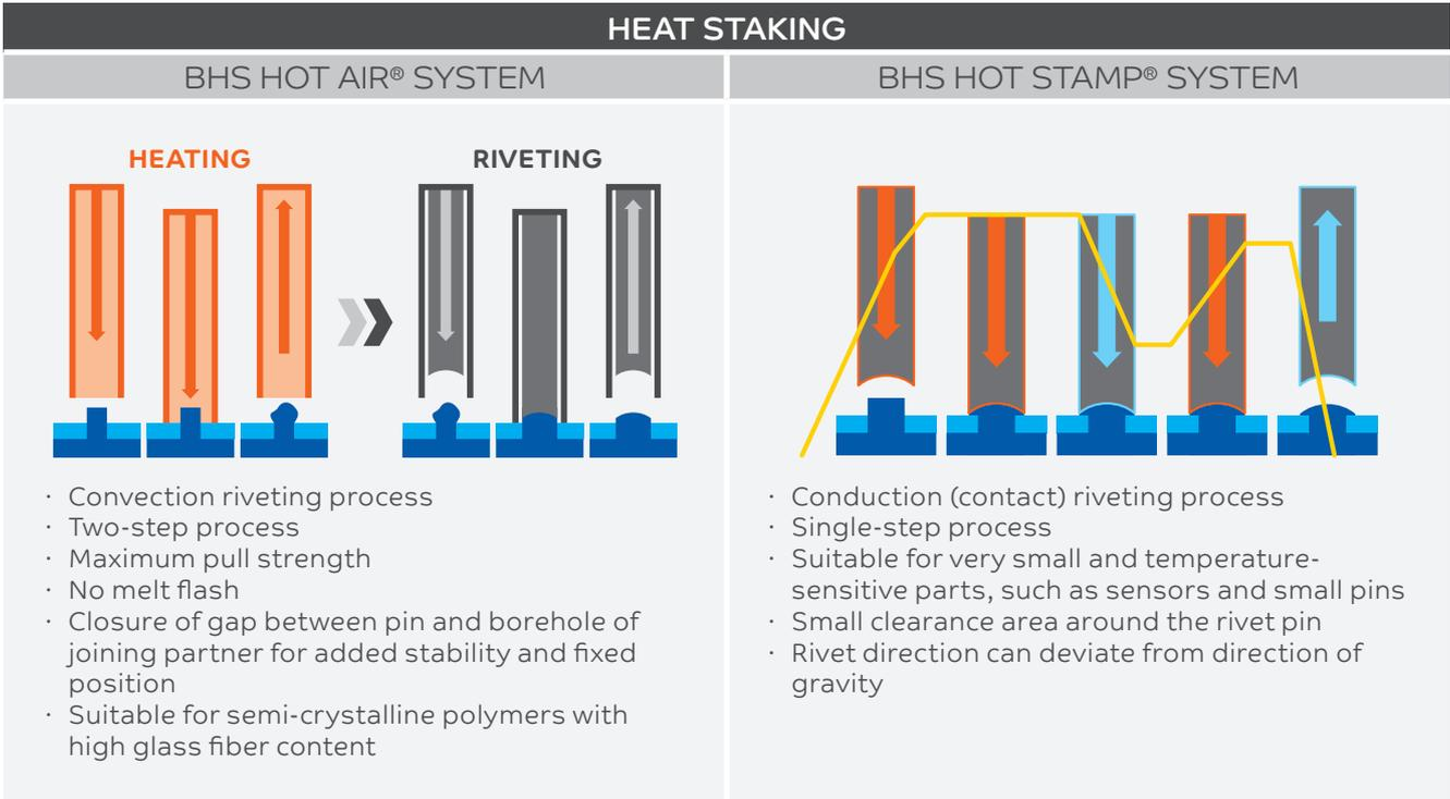
**Figure 4.** Comparison of BHS HOT AIR® with BHS HOT STAMP® heat staking methods
