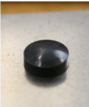
**Figure 5.** Rivet head before pull force test with BHS HOT AIR® System
