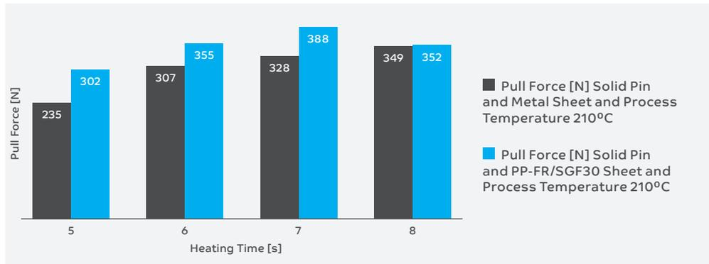
**Figure 6.** Test results for BHS HOT AIR® System
