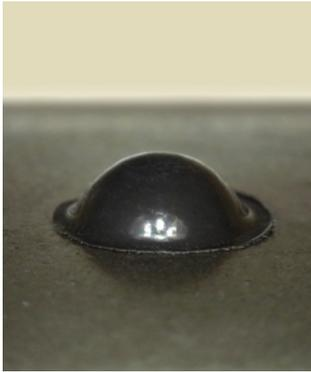
**Figure 7.** Rivet head before pull force test with BHS HOT STAMP® System
