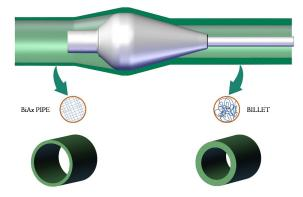
SABIC has developed a new range of PE and PP resins that offer significant improvements in key performance properties for biaxially stretched pressure water pipes.
