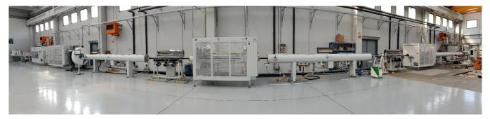
SABIC introduces unique new BiAx pipe technology in collaboration with major players in the pipe industry. The photo shows an integrated system from Tecnomatic for continuous BiAx pipe extrusion, with dedicated new high-performance PE and PP resin formulations from SABIC.
