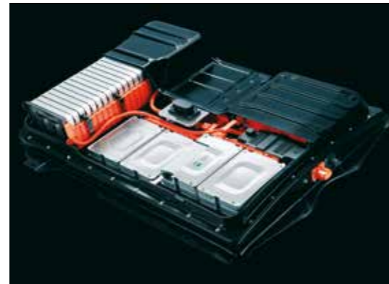
SABIC's hybrid plastic/metal battery protection solution helps improve battery protection performance while cutting weight by up to 40 to 60 percent.
