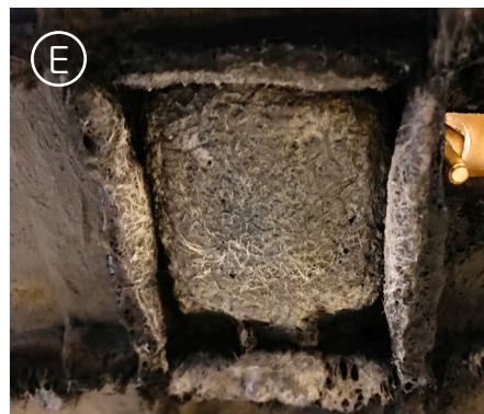
A view of the post-test plaque after the flame test shown in D
