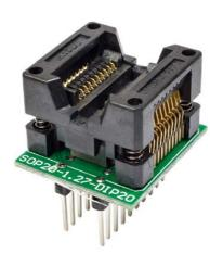
BiTS are critical devices that enable IC testings prior to the PCB final assembly in order to minimize early failures and increase the reliability and lifetime of the final devices.
