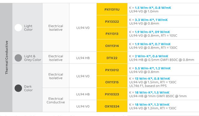
\* Thermal conductivity measured with Hotdisk TPS2500 In-plane with a 3mm plate (60 by 60mm, film-gated). Non-brominated, non-chlorinated, flame retardant system DTK: PC based
