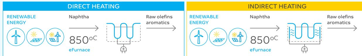
By using electricity from renewable sources instead of natural gas, electric steam cracker furnaces, one of the most energy-intensive production processes, can potentially reduce CO<sub>2</sub> emissions by at least 90% compared to conventional technologies. The electricity-based heating concepts for olefin production, which will be tested at the plant in the future, require a total of 6MW of renewable energy.
