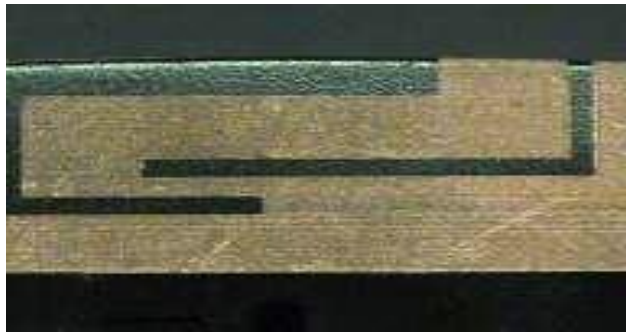
After copper strike Strike time:15-30min
