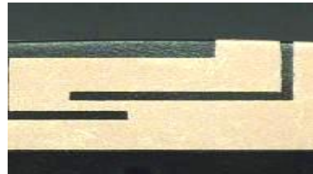
After copper build Rate:>12um/2-4 hrs
