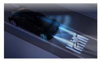
The digital matrix LED headlight could project safety or warning images in front of a car to improve safety and security for both drivers and pedestrians.
