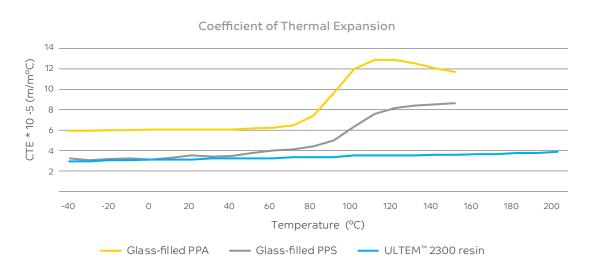
Compared with glass-filled PPA and glass-filled PPS, ULTEM resin keeps a low and stable CTE between -40°C to 200°C and maintains better dimensional stability over a wide temperature range.
